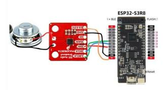
Refer to the below photo: it is possible to solder the DAC directly to the ESP32 in the following way (the pins are already aligned)
