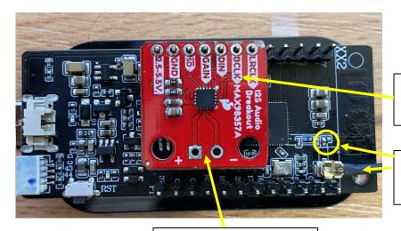
DAC+AMP Solder that way, no need for wires
